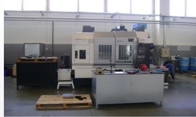
CNC milling machine OKUMA GENOS, 2015 , 3 AXIS Table travel : X=1050; Y=560; Z=460
