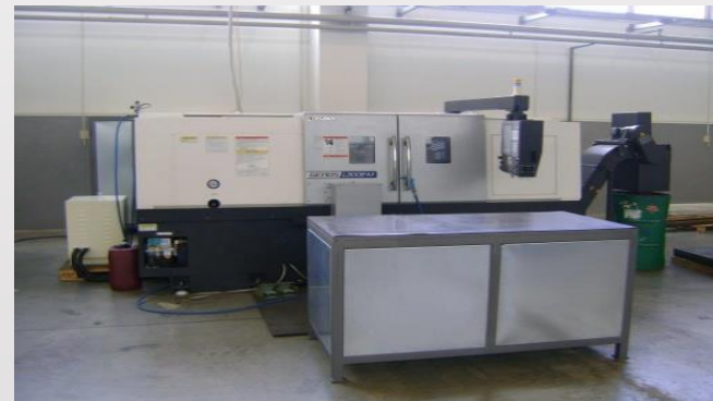
CNC lathe OKUMA Type: GENOS L300E-M Max Dimensions: 500x1140
