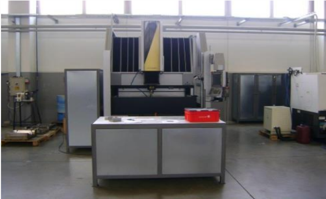
EDM (Electrical discharge machine / Erozimat ) SODIC, 2016 1400x950x500 working space Table travel (X x Y x Z): 850x850x420
