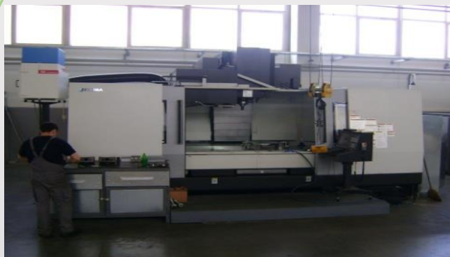
CNC milling machine OKUMA MILLAC, 2016 Table travel: X=2050; Y=850; Z=750
